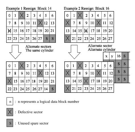
Figure 3.8 Alternate block allocation by REASSIGN BLOCKS command
